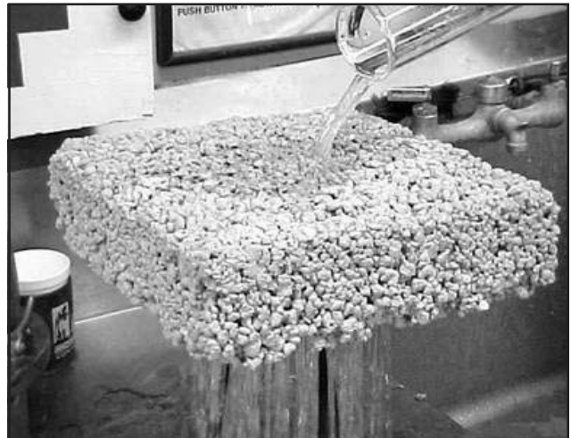
Pervious Concrete permits storm water to percolate
